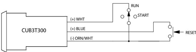
A machine shop manager charges customers for machine time by the hour. He is also interested in tracking machine run time vs. down time. A CUB3T310 connected across the 115 VAC spindle motor of a drill press will serve both purposes. A reading taken before and after each job will indicate the actual machine run time in tenth hour increments. A reading at the beginning and end of each shift will indicate total run time, allowing the manager to evaluate production efficiency and down time.
