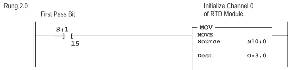
Figure 8.3 Program to Convert °F to BCD
