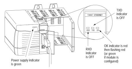
The following table describes the displays of the transmit (TX) and receive (RX) indicators:
