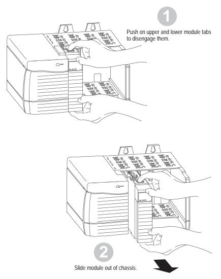
If you are replacing an existing Ethernet module with an another Ethernet module, and you want to resume identical system operation, you must install the new Ethernet module in the same slot.
