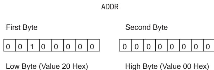
**Important:** PLC and PLC-2 Family controllers use this same logical addressing format when they transmit command messages to another station. If you plan to transmit a command message to your computer from one of these PCs, you should set up a buffer space in your computer to simulate PC memory. You would then have to write computer application programs to accept and execute commands from the PC stations and to translate the ADDR value into the corresponding address in the simulated PC memory.
