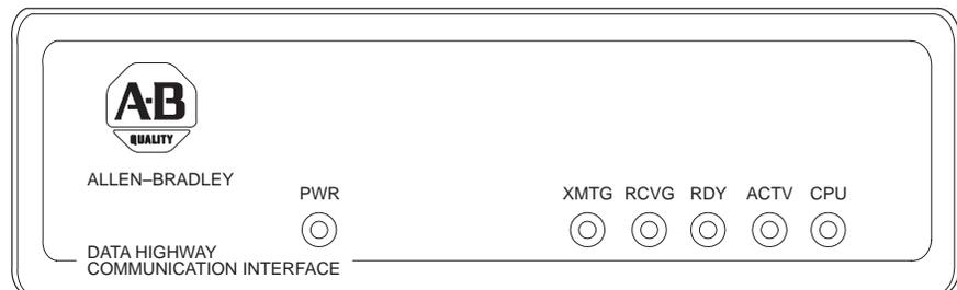
The XMTG light comes on when the KF2 module is current master of the network link and is transmitting a command or reply message.
