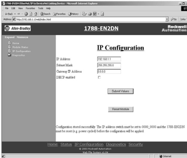
The IP address can be set with the web page only if the linking device already has a valid IP address. Typically, you can do this by using the DIP switch to force the linking device to use a temporary IP address after you cycle power. To configure the IP address with the web page:
