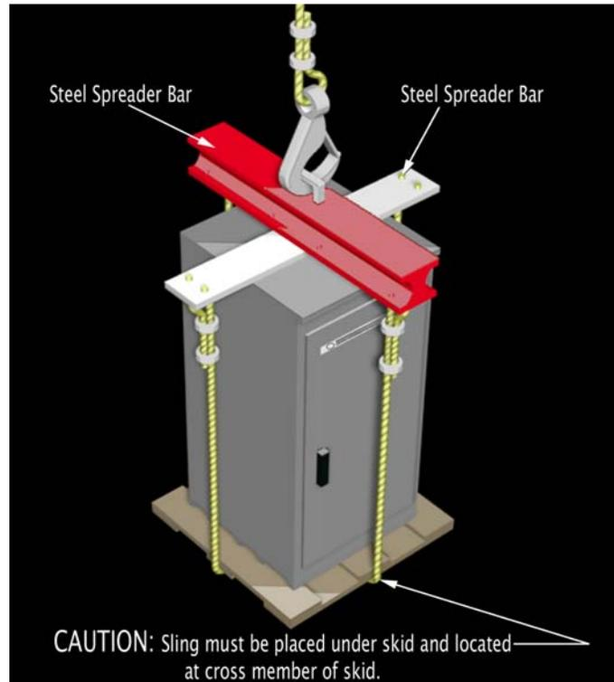
Figure 5 Lifting sling on NEMA Type 3R motor control center without lifting angle
