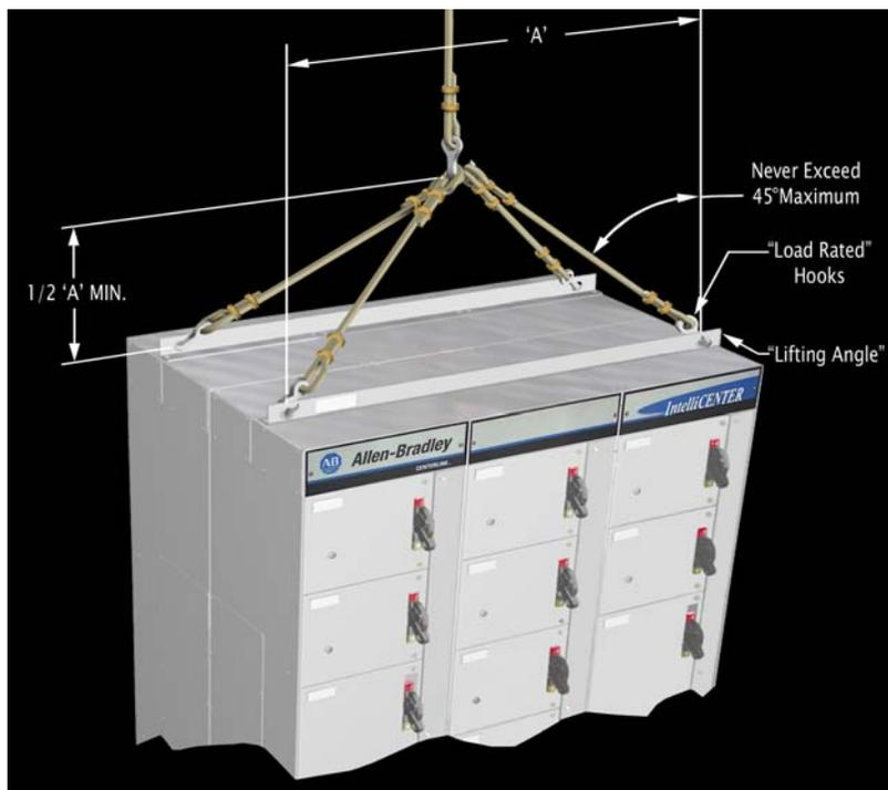
Figure 3 Overhead lifting a motor control center with back-to-back construction
