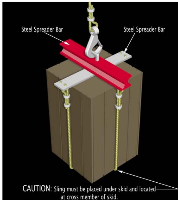
Figure 4 Lifting sling on export packaged motor control center
