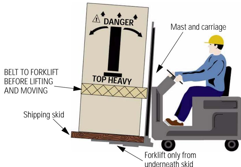
**Figure 1 Forklifting a standard motor control center**
