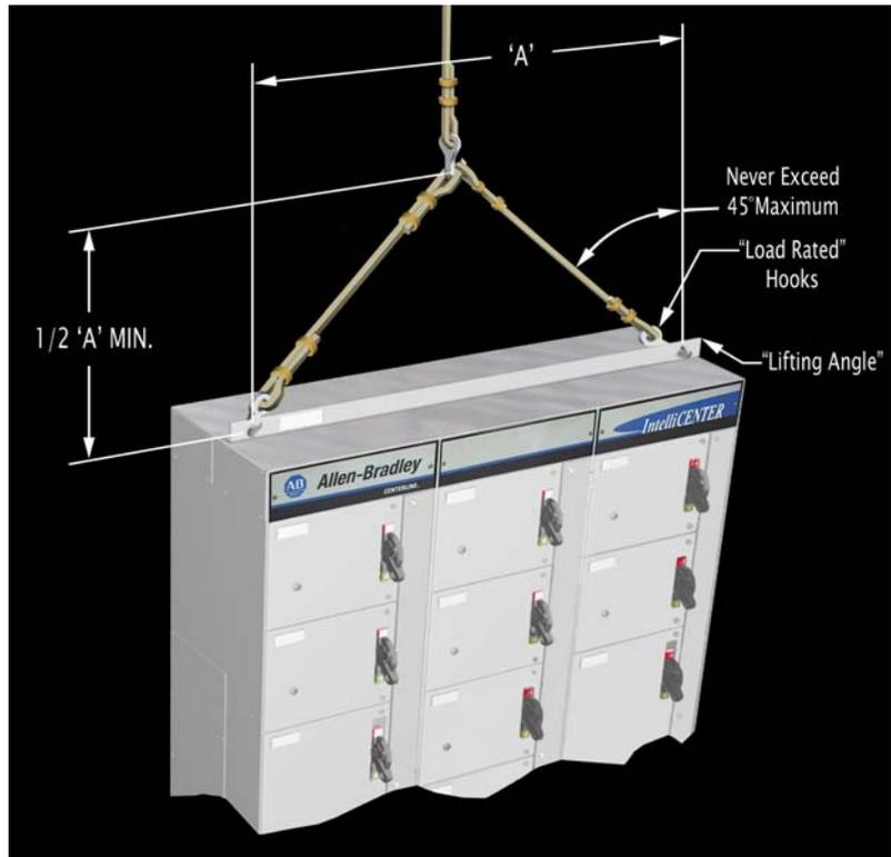
Figure 2 Overhead lifting a front mounted motor control center
