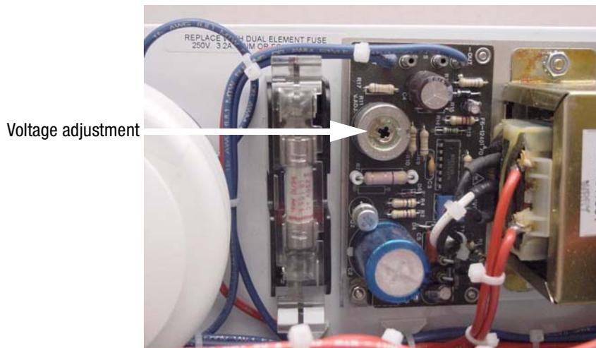
**Figure 2 DC voltage adjustment**
