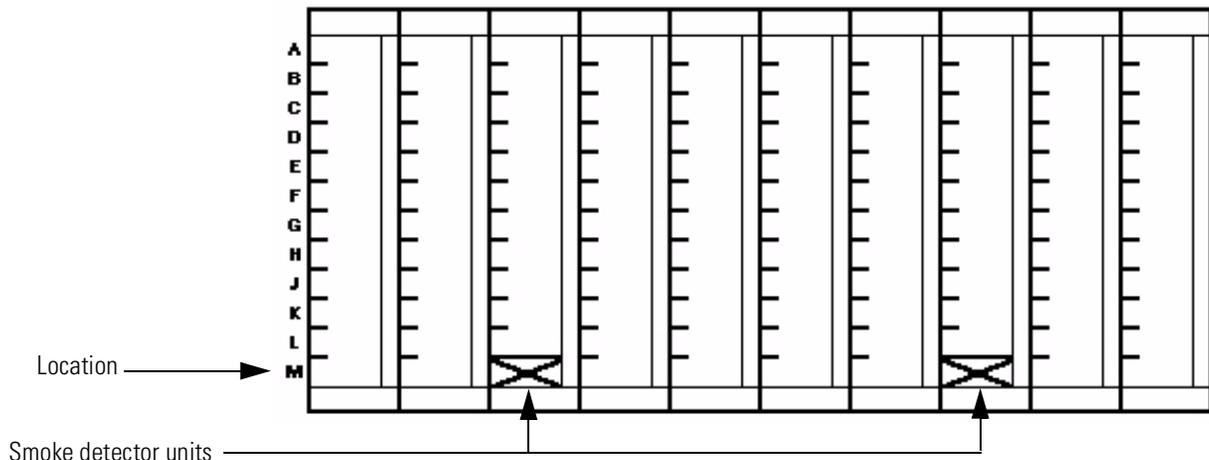
**Figure 1 Correct placement of smoke detector units**
