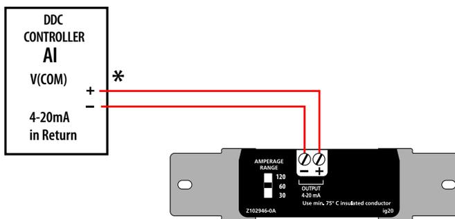
\*A resistor can be added in parallel to convert the 4-20mA signal to a VDC signal 250 ohm = 1-5VDC 500 ohm = 2-10VDC
