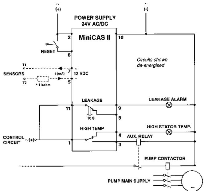
\*) Fit resistor to avoid short circuit if only thermal contacts are to be connected.
