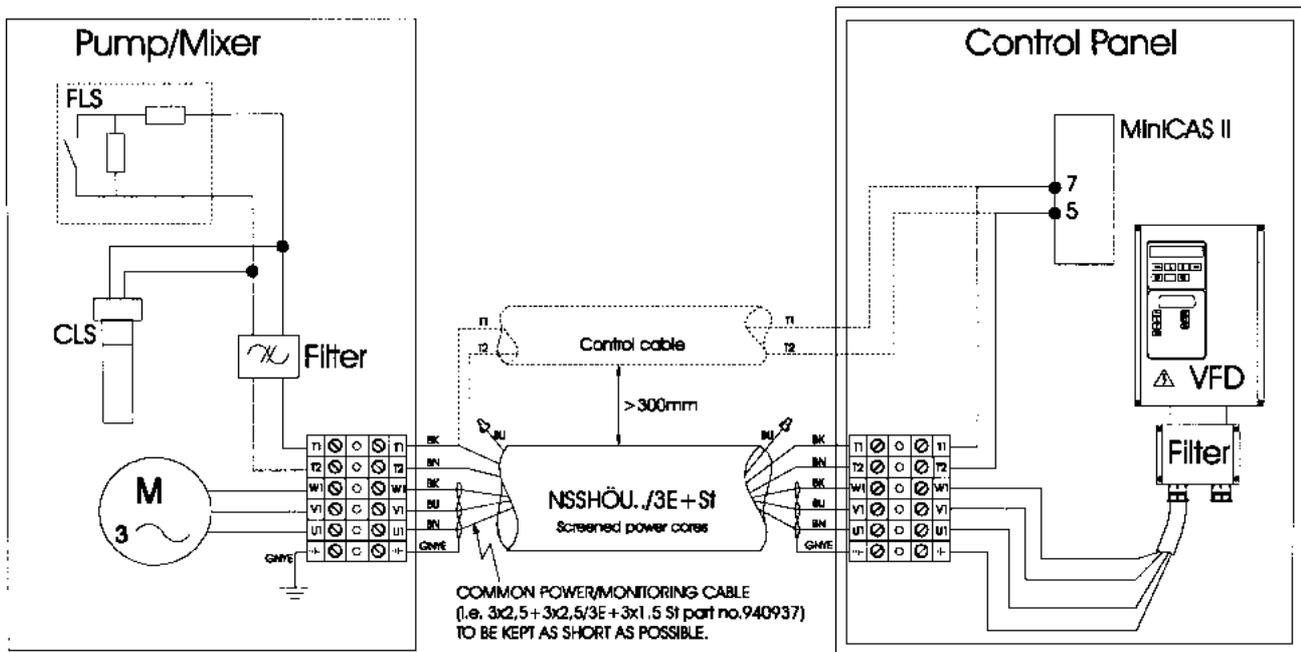
In installations utilising variable frequency inverters for speed control of pumps, interference from a variable frequency drive (VFD) may cause nuisance tripping of monitoring equipment and the electronic sensor CLS.
