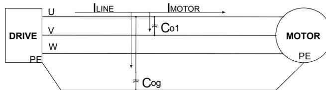
Capacitively coupled currents could exceed the drive rating.
