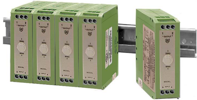
Transducer output is derived from the average absolute value of the input and calibrated as the RMS value of a sine wave input.
