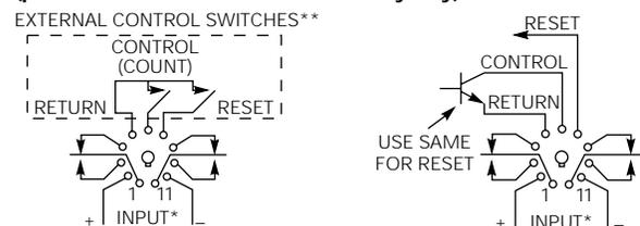
\* **Note:** Input polarity for DC operation. For most reliable operation on AC, connect high side to "+" and low side to "-".
